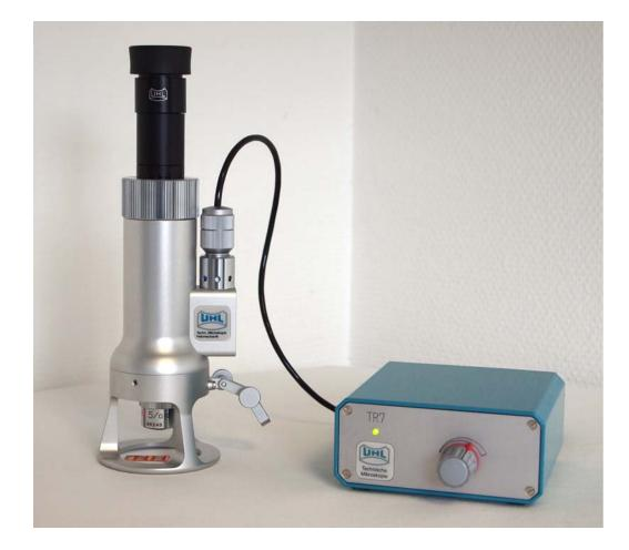
Portable measuring microscope with coaxial and angular incident illumination of high quality.
